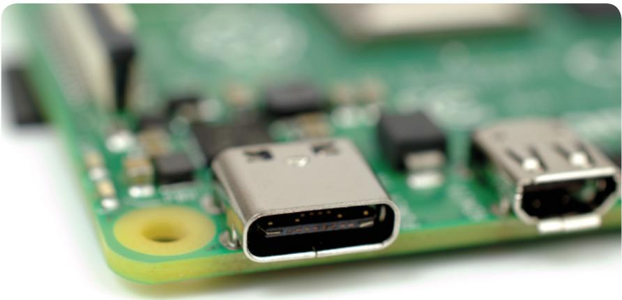
▲ **Figure 1-11:** Raspberry Pi's USB Type-C power port
