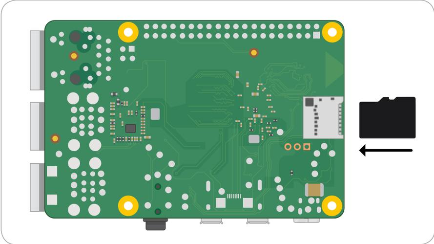
The microSD card will slide into the connector, then stop without a click.
