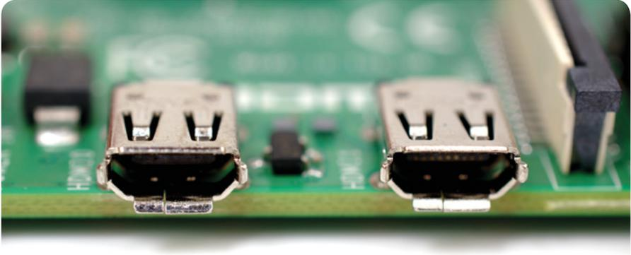
▲ **Figure 1-10:** Raspberry Pi's micro-HDMI ports
