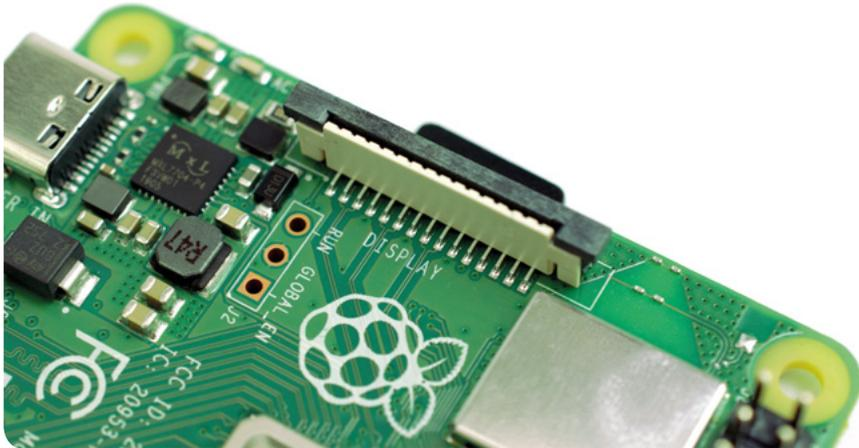
▲ **Figure 1-12:** Raspberry Pi's display connector (DSI)
