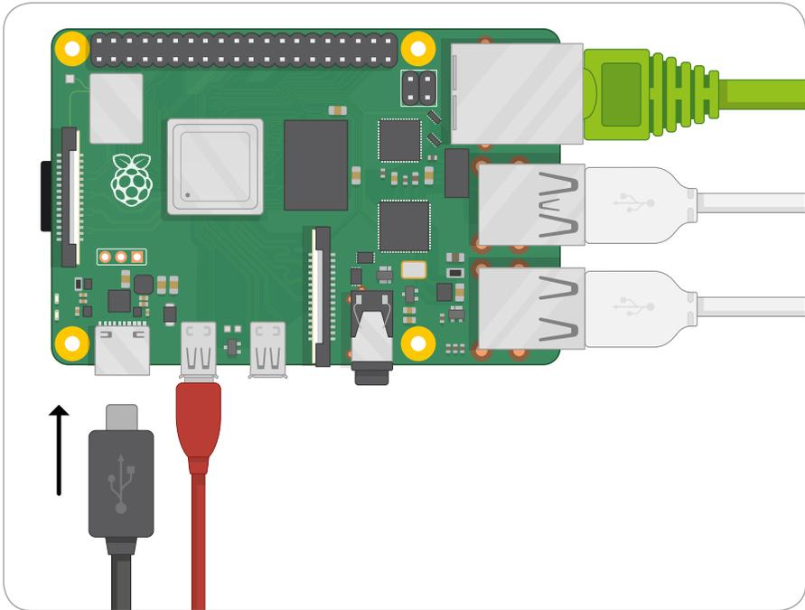
Finally, connect the power supply to a mains socket and switch the socket on; your Raspberry Pi will immediately start running.
