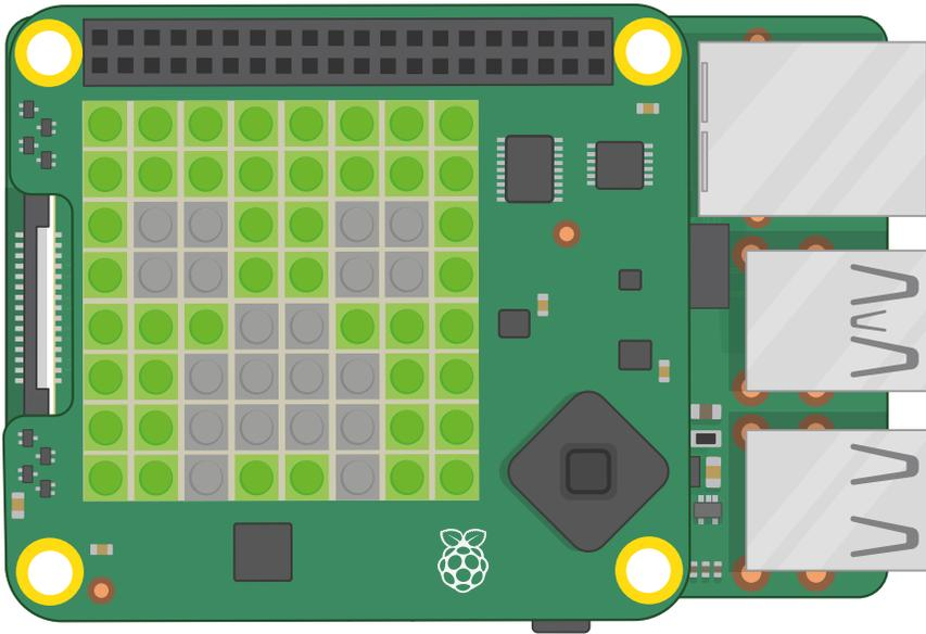
▲ **Figure 7-15: Displaying an image on the matrix**
