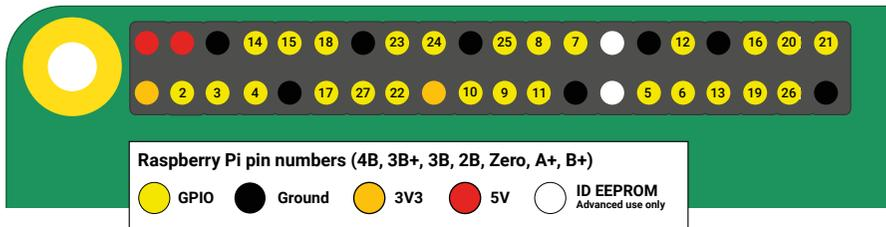
Raspberry Pi's GPIO header is made up of 40 male pins. Some pins are available for you to use in your physical computing projects, some pins provide power, while other pins are reserved for communicating with add-on hardware like the Sense HAT (see **Chapter 7**).
