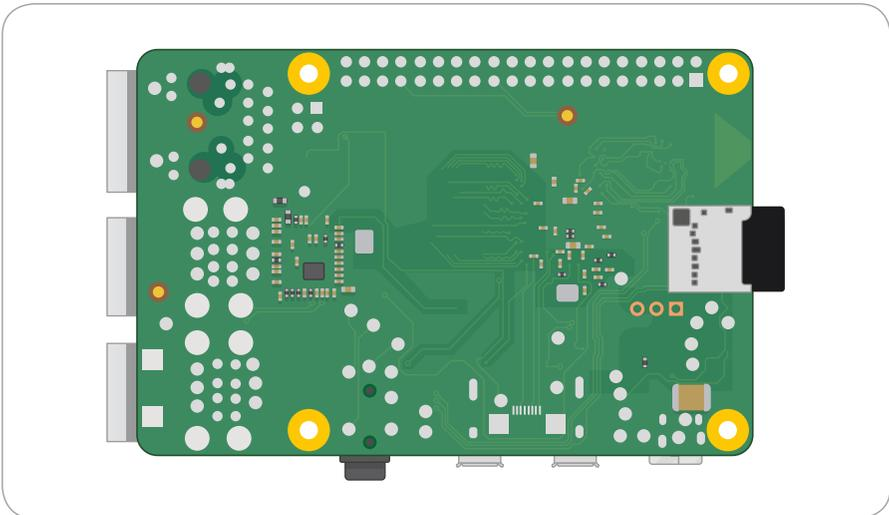
If you want to remove it again in the future, simply grip the end of the card and pull it gently out. If you're using an older model of Raspberry Pi, you'll need to give the card a gentle push first to unlock it; this isn't necessary with a Raspberry Pi 3 or 4.
