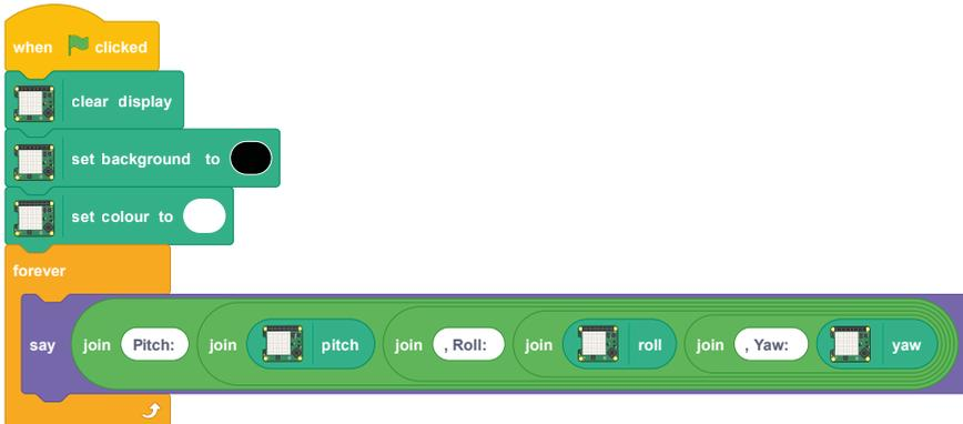
Click the green flag to run your program, and try moving the Sense HAT and Raspberry Pi around – being careful not to dislodge any cables! As you tilt the Sense HAT through its three axes, you'll see the pitch, roll, and yaw values change accordingly (**Figure 7-25**).
